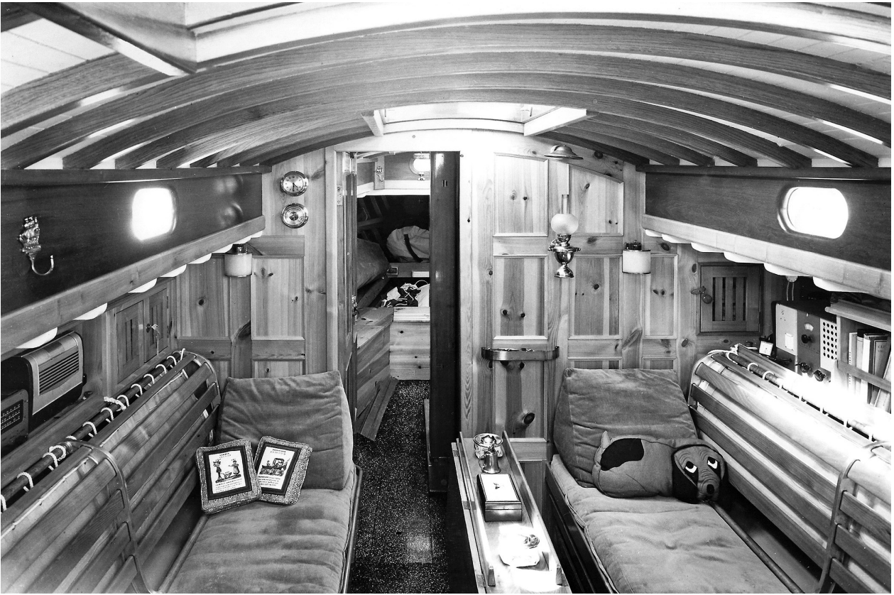
Above: Interior view of #32 PRISCILLA (now MIRAGE), built in 1955. Along with the endearingly droll “sad puppy” pillow, details of interest include the spatter-painted cabin sole, multiple beanbag ashtrays, and vintage electronics. There is no cabin heater.
