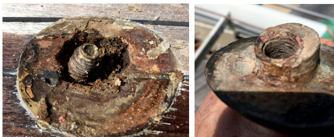
Left, bronze rod top, right, backstay fitting, both with corroded threads.
