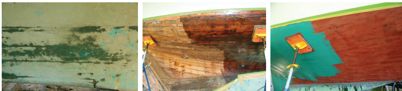
Left to right: Golondrina's bottom at the start; woodwork done and half primed with penetrating epoxy; one coat of red followed by the first coat of green.
