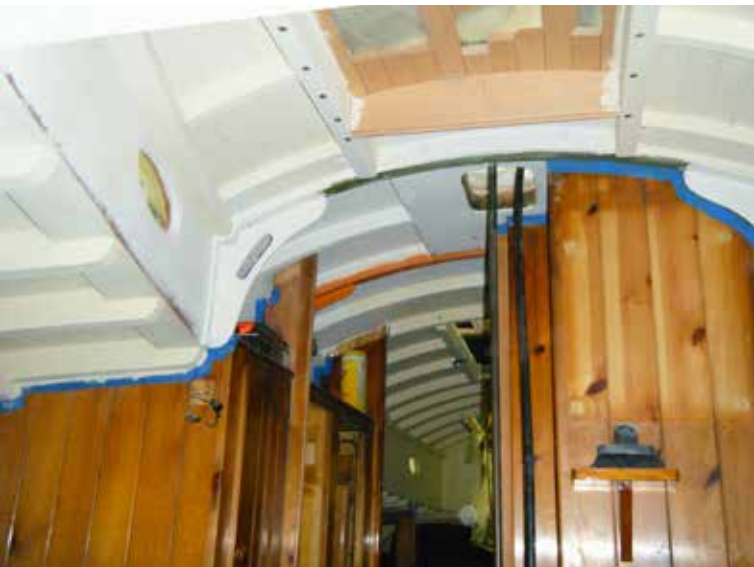
Main Cabin primed. Note the custom SS reinforcing brackets, with hand hold.
