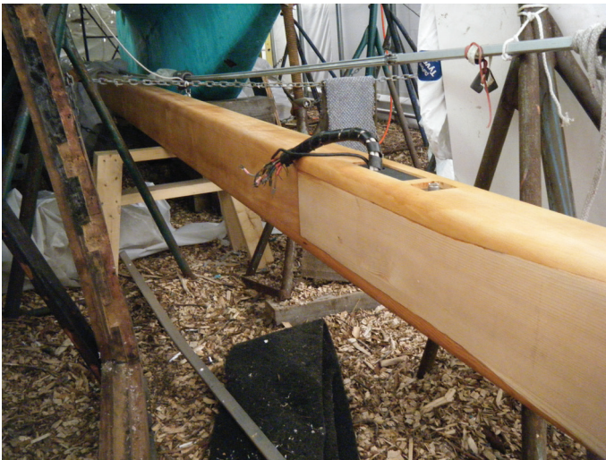
The damaged base of the main mast has had new wood scarfed in. The booms and mizzen were not salvageable and new spars are being built.
