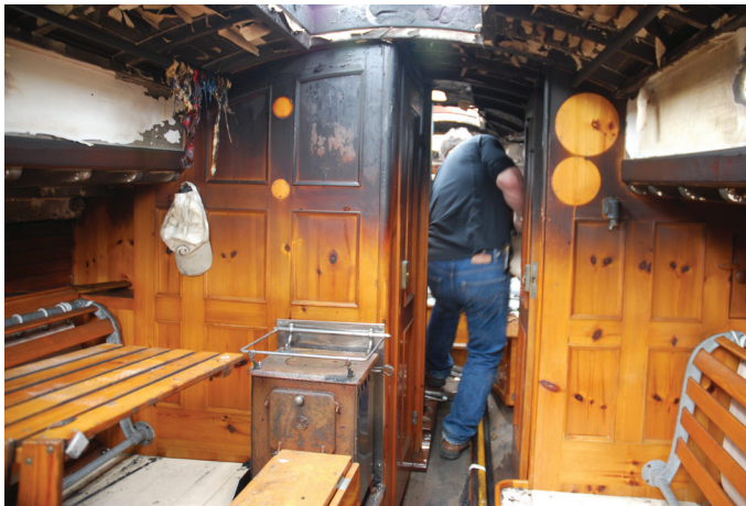
Don inspects Abaco before purchase, where you can see the fire damage. The fire started behind the galley stove, then a flashover blew out the three hatches, igniting the sails and spars. Molten Dacron fell on the house, deck and cockpit where most of the damage occurred.
