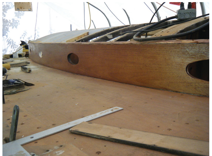
The starboard cabin side has been veneered to cover the charring. Burned sections of the deck have been cut out and replaced
