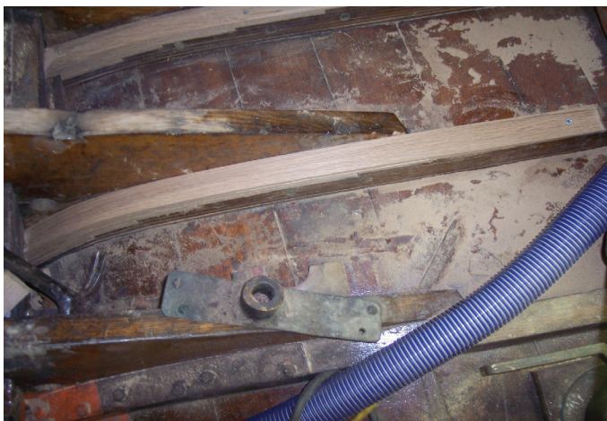
While the cockpit is out, the delaminated frames and floors are being repaired.
