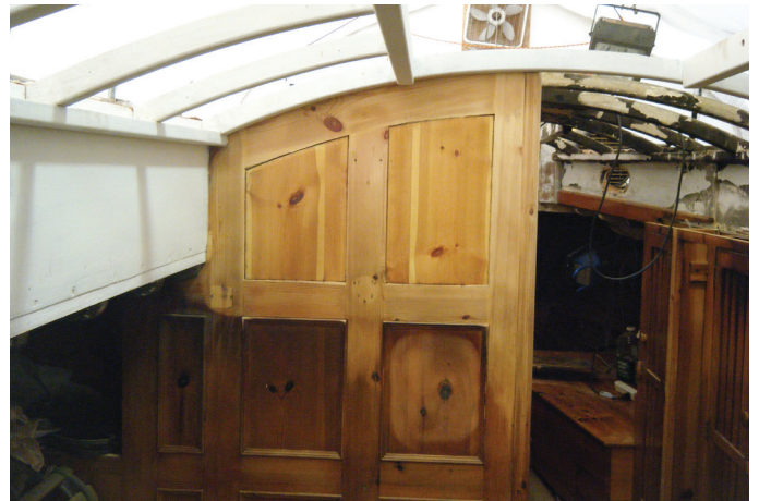
Don has begun to clean up the charred bulkheads and is replacing or repairing each house beam.
