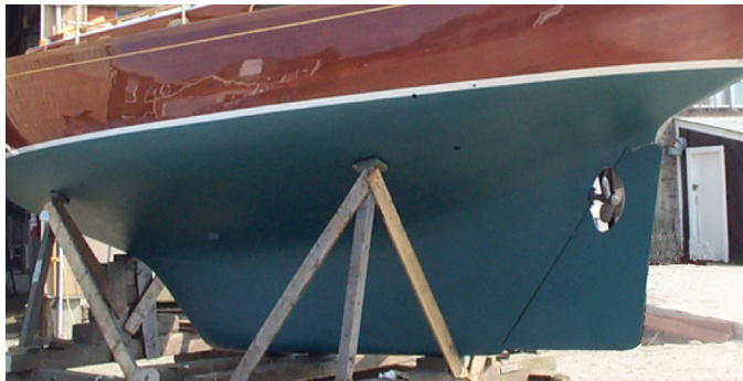
The triangular rudder, unique to Coriolis, and cutaway keel are visible here.
