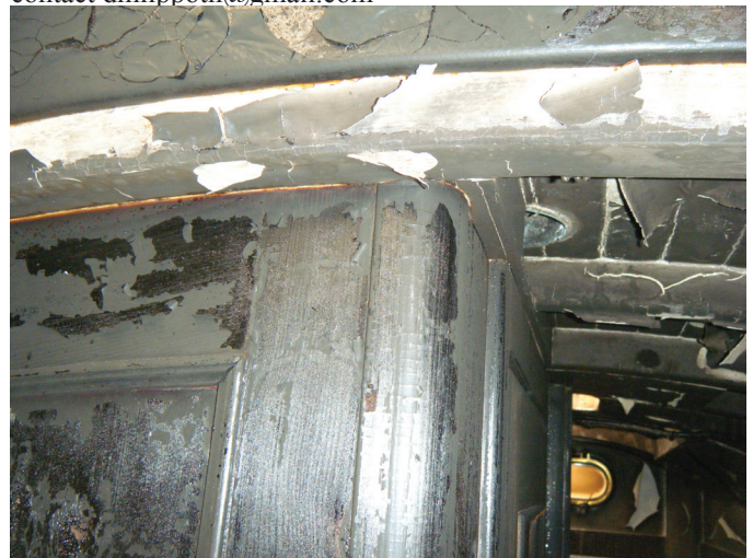
Abaco's varnished and painted interior, after the fire.
