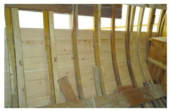
couraged but we pushed on. We decided to laminate new oak frames to replace or sister all the frames as necessary throughout the hull. We removed the sheer strake, the toe rail and the outer most plank of the deck to expose the tops of the frames. We replaced quite a few entire frames and sistered others with new laminated oak replacements.
