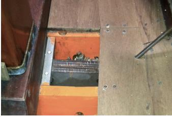
Above is the beam, made up of four layers of 1/2" stainless steel, installed on GOLONDRINA. The 1/2" rod, on the right, ends in a Navtec eye pinned between the ss plates. All the parts you see were installed through that opening in the floorboards. There is no rust even after 15 years and two trips to the Caribbean.
